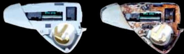
These two devices have been put through weeks of extreme environmental testing. The device on the left is protected with iSolate™ nanotech. No damage was observed on this device. The non-coated device on the right is visibly corroded.
